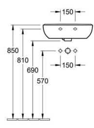
Note: All dimensions are in millimetres and are subject to normal manufacturing variations. Always use the physical product measurements for cut-outs and rough-ins as the technical details shown may differ from the actual product. Use acetic cured silicone sealant. Do not use epoxy type adhesives. Clean with damp cloth. Do not use abrasive cleaners, liquids or pastes.
