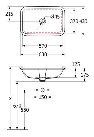
Note: All dimensions are in millimetres and are subject to normal manufacturing variations. It is reccommended to use the physical product measurements for cut-outs and rough-ins as the technical details shown may differ from the actual product. Use acetic cured silicone sealant. Do not use epoxy type adhesives. Clean with damp cloth. Do not use abrasive cleaners, liquids or pastes.
