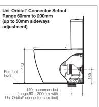
**Wall Faced Close Coupled Toilet Suite with Chrome** Cistern Button and Seat with Stainless Steel Seat Caps Code No. 4.5/3 litre Back Entry Internal Overflow with inVogue Soft Close Quick Release Seat 746350 4.5/3 litre RH Bottom Inlet Internal Overflow with inVoque Soft Close Quick Release Seat 746250
