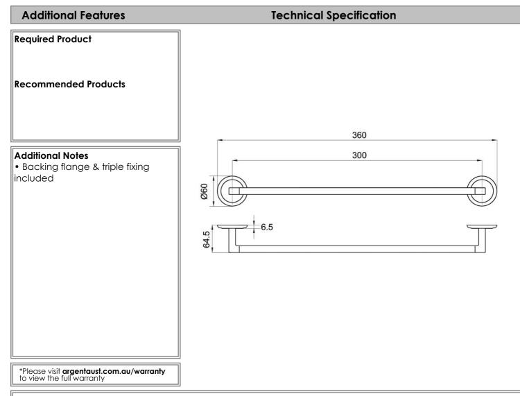
Note: All dimensions are in millimetres and are subject to normal manufacturing variations. It is reccommended to use the physical product measurements for cut-outs and rough-ins as the technical details shown may differ from the actual product. Use acetic cured silicone sealant. Do not use epoxy type adhesives. Clean with damp cloth. Do not use abrasive cleaners, liquids or pastes.
