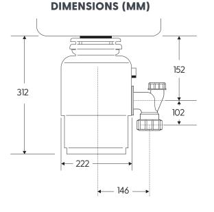
Type of Feed Continuous On/Off Control Wall Switch or Built-In Air Switch Single Phase **Power Supply** Auto-Reverse Reversing Grind System Time Ratina Intermittent Lubrication Permanently Lubricated Upper & Lower Bearings Shipping Weight 8.8 kg (Approx.) Unit Finish Black Enamel Grey TEN-1706 Overall Height 312 mm Grind Technology 2-Stage Grind Technology
