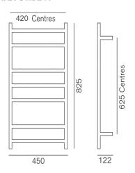
MEASUREMENTS SUBJECT TO MANUFACTURING TOLERANCE
