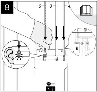
\* NOTICE: Property Damage. Pinched or blocked water lines may cause damage to the water tank. Check to make sure tubes are connected correctly and are pushed down as far as possible.
