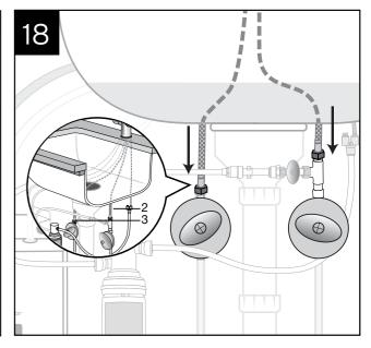
\* NOTICE: Property Damage. Tube runs need to form to the cabinet's contours to allow storage space with no sharp bends. Tubes need clean, perpendicular, burrfree cuts to ensure a true fit. Join remaining tube to cold water supply only. Note: Check all connections to ensure they are tight and that there are no leaks.
