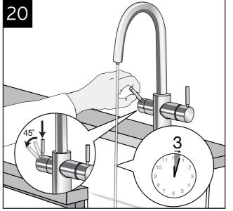
**Note:** Water will be cold at first. Allow 12-15 minutes for water to reach target temperature. Gurgling or hissing is normal during the initial heating cycle.
