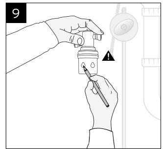
WARNING. (Personal Injury) Do not locate filter above an outlet or other electrical device. Install head and bracket so that connections require no stretching, kinking or pinching of tubing.
