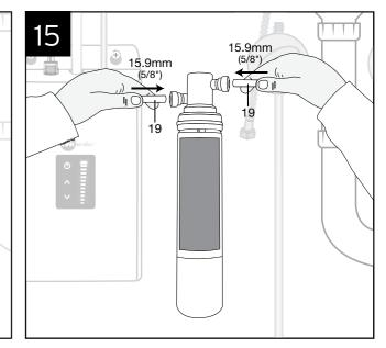
\* NOTICE: Property Damage. Top surface of cartridge will be flush with bottom of filter head when fully engaged.
