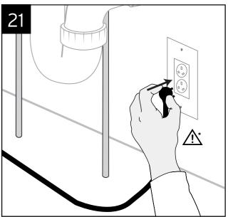
\* NOTICE: Property Damage. Do not use an extension lead with the tap. (A standard earthed outlet within 760 mm (30") of the tap is required under the sink.)
