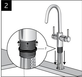
\* NOTICE: Property Damage. Do not pinch or break copper tubing. Do not distort Note: Required 33.5 mm (1.3") hole size. For ease of installation put the
