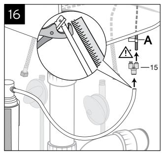
\* NOTICE: Property Damage. Do not extend the lines farther than the 400 mm (16") provided. Ensure tube(s) and "Y" connector fit securely.
