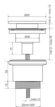
Note: All dimensions are in millimetres and are subject to normal manufacturing variations. Always use the physical product measurements for cut-outs and rough-ins as the technical details shown may differ from the actual product. Use acetic cured silicone sealant. Do not use epoxy type adhesives. Clean with damp cloth. Do not use abrasive cleaners, liquids or pastes.
