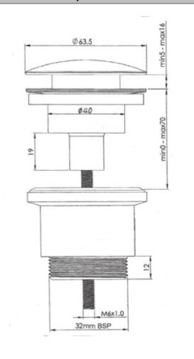
Note: All dimensions are in millimetres and are subject to normal manufacturing variations. Always use the physical product measurements for cut-outs and rough-ins as the technical details shown may differ from the actual product. Use acetic cured silicone sealant. Do not use epoxy type adhesives. Clean with damp cloth. Do not use abrasive cleaners, liquids or pastes.
