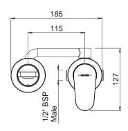
**CONSTRUCTION**: Eco Brass **CARTRIDGE TYPE**: Ceramic
