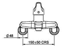
CONSTRUCTION: Brass body CARTRIDGE TYPE: Ceramic (SP033550) CLASSIFICATION: Suitable for all pressure systems INLET CONNECTIONS: 1/2 " BSP Female WORKING PRESSURE: 35 - 500kPa DIMENSIONS FOR FITTING: 150±50mm distance between connectors OPERATING TEMPERATURE: 5 °C - 80 °C
