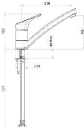
CONSTRUCTION: Brass body CARTRIDGE TYPE: Ceramic (SP033510) CLASSIFICATION: Suitable for all pressures INLET CONNECTIONS: 1/2 " BSP Female WORKING PRESSURE: 35 - 500kPa DIMENSIONS FOR FITTING: 35 mm diameter hole OPERATING TEMPERATURE: 5 °C - 80 °C WATER FLOW RATE: 9.0 l/m low pressure - 8.0 l/m high pressure
