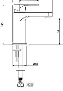
**CONSTRUCTION:** Brass body CARTRIDGE TYPE: 25 mm ceramic SUPPLY: Suitable for mains pressure only INLET CONNECTIONS: 1/2 " BSP Female WORKING PRESSURE: 150 - 1000kPa DIMENSIONS FOR FITTING: 35 - 38 mm diameter hole
