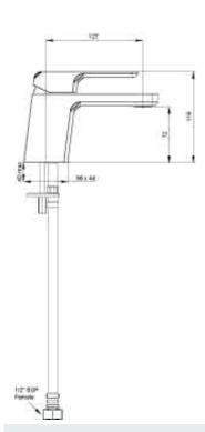
**CONSTRUCTION:** Brass body **CARTRIDGE:** Ceramic
