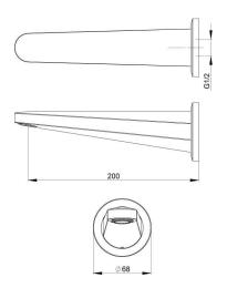
CONSTRUCTION: Brass body PROJECTION: 200mm CLASSIFICATION: Suitable for all pressure systems PIPE CONNECTION: 1/2 " BSP Female WORKING PRESSURE: above 35 kPa OPERATING TEMPERATURE: 5 °C - 80 °C
