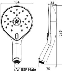
CONSTRUCTION: Chrome-plated CLASSIFICATION: Suitable for all pressure systems INLET CONNECTIONS: 1/2 " BSP Male WORKING PRESSURE: 35 - 500kPa OPERATING TEMPERATURE: 5 °C - 70 °C
