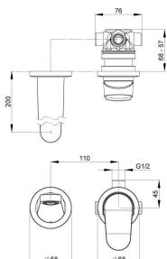
CONSTRUCTION: Brass body CARTRIDGE: Ceramic (SP033510)
