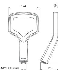
CONSTRUCTION: Chrome-plated CLASSIFICATION: Suitable for mains pressure only INLET CONNECTIONS: 1/2" BSP Male OUTLET CONNECTION: N/A WORKING PRESSURES: 100 - 500kPa OPERATING TEMPERATURE: 5 °C - 65 °C WATER FLOW RATE: 7.5 l/m
