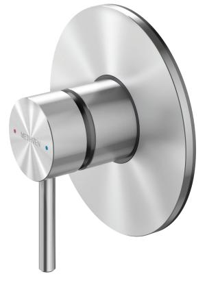
CONSTRUCTION: Stainless steel, brass and plastic CARTRIDGE TYPE: Ceramic CLASSIFICATION: Suitable for mains/high pressure only INLET CONNECTIONS: 1/2" BSP Male OUTLET CONNECTIONS: 1/2" BSP Male WORKING PRESSURE: 150 - 1000kPa OPERATING TEMPERATURE: 5 °C - 80 °C
