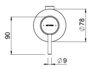
CONSTRUCTION: Stainless steel, brass and plastic CARTRIDGE TYPE: Ceramic CLASSIFICATION: Suitable for mains/high pressure only INLET CONNECTIONS: 1/2" BSP Male OUTLET CONNECTIONS: 1/2" BSP Male WORKING PRESSURE: 150 - 1000kPa OPERATING TEMPERATURE: 5 °C - 80 °C
