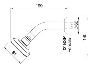
CONSTRUCTION: Brass arm CLASSIFICATION: Suitable for all pressure systems INLET CONNECTIONS: 1/2 " BSP Female WORKING PRESSURE: 35 - 500kPa OPERATING TEMPERATURE: 5 °C - 70 °C WATERFLOW RATE: 9.0 l/m
