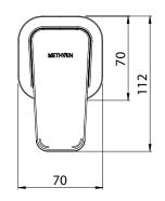
CONSTRUCTION: Brass body CARTRIDGE: Ceramic CLASSIFICATION: Suitable for mains pressure only INLET CONNECTIONS: 1/2 " BSP Male OUTLET CONNECTIONS: 1/2 " BSP Male OPTIMUM PRESSURE: 150 - 500kPa OPERATING TEMPERATURE: 5 °C - 80 °C
